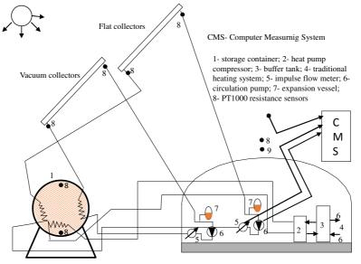
Fig. 1. Schematic representation of measurement stand
