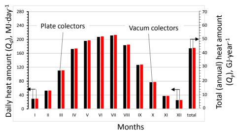
Fig. 4. Daily and annual amount of heat in discussed system with plate and vacuum solar collectors
