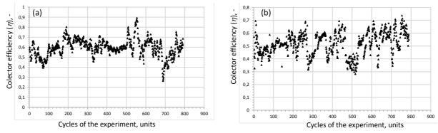
Fig. 2. Efficiency of analysed collectors: a - plate; b - vacuum
