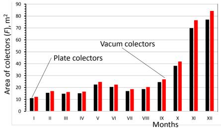
Fig. 3. Required surface area of solar collectors for irrigation of plants
